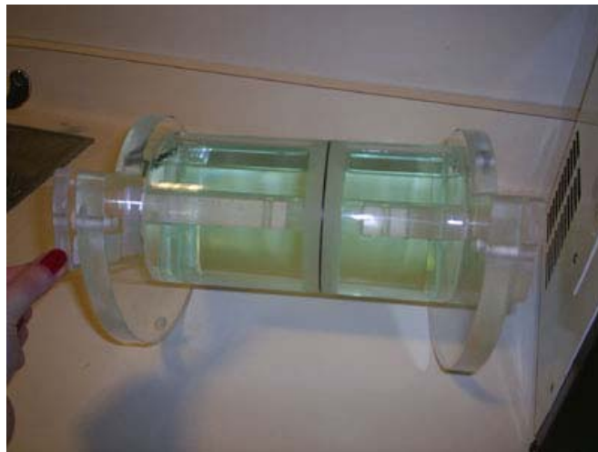
Figure 3: A phantom commercially available for use with an MR imager [photo taken by the authors]
