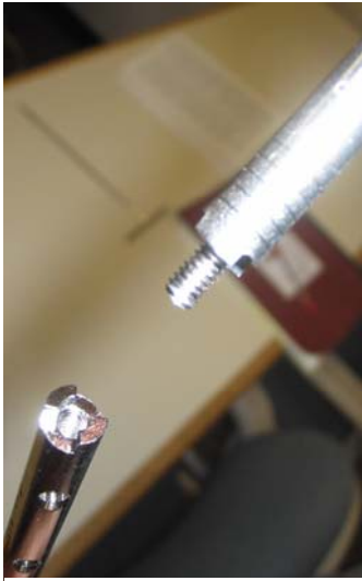
Figure 2: Nail head (lower left) and extension joint (upper right).
