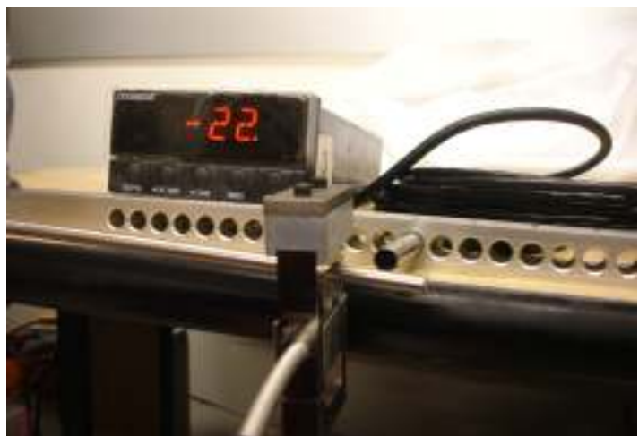
Figure 11: Testing setup. The force gauge pulls down on the nail until the entire hole in the drill guide sleeve can be seen. The picture depicts the point at which the force would be recorded.
