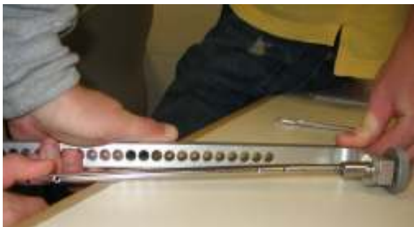
Figure 1: The nail and extension are secured to the jig. The nail can be seen deviating from the jig holes at the extension-nail joint.
