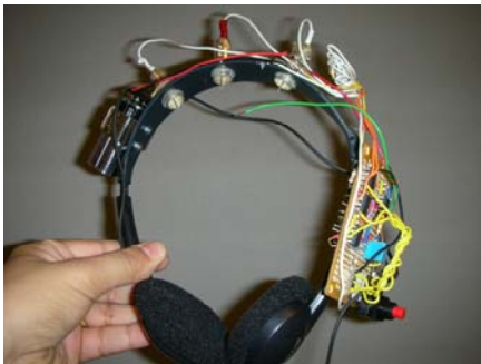
Figure 3. Integrated prototype with electrodes, amplifier, and battery power source.
