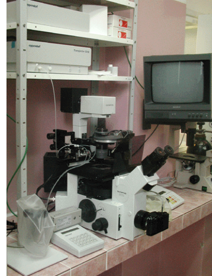
Fig. 1 – Micromanipulator set-up with integrated analog monitoring equipment.
