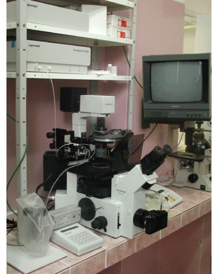
Fig. 1 – Micromanipulator set-up with intergrated analog monitoring equipment.
