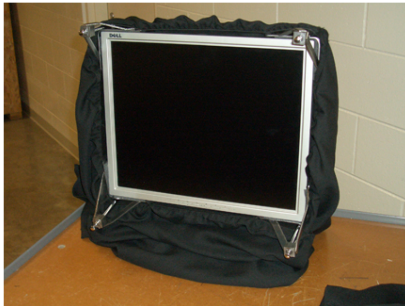
Figure 2. The front side with corner pieces, contracted extenders, and primary hood shown
