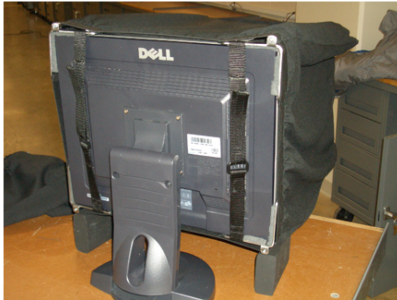
Figure 1. The back side with the block supports, corner pieces, straps, and primary hood shown
