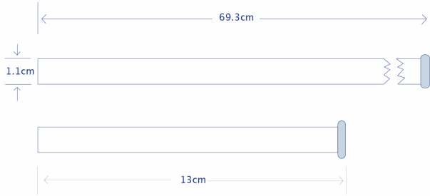
Extension pieces: Top: Extended. Bottom: Contracted
