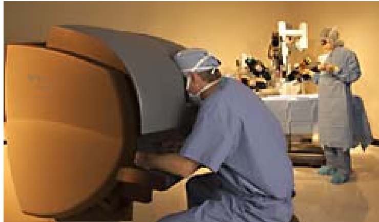
Figure 1: da Vinci ® Surgical System allows surgeons to operate from across the room.
