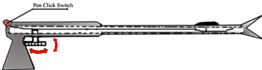
Figure 5: Trigger Controlled surgical forceps. This design allows synchronized shaft bending and rotating which closely replicates human wrist maneuvers. The red “pen click” switch located on the top of the handle allows for locking the graspers in the open or closed position.
