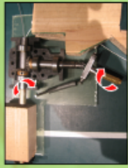
Figure 5: Section of Assembled Grip Mechanism to shaft
