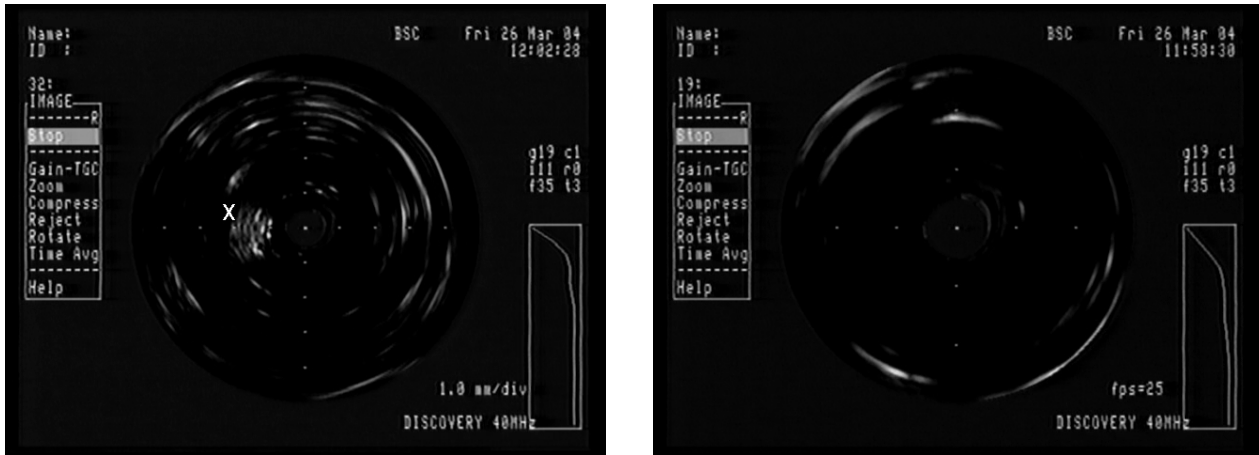
Figure 7. Ultrasound gel with probe alone in hollow plastic tube without simulated calcification (left) and with simulated calcification (X) (right). The profile of the hollow plastic tube is visible near the edge of each image.
