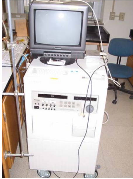
Figure 8. Ultrasound machine at Medical Physics Department on UW-Madison campus used for initial testing of IVUS probes with phantoms. Data will be recorded on VHS and digitally captured.
