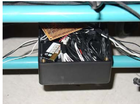
Fig. 14 The control box of the circuit houses the circuit board, coiled wire, and the 9V power source. It is mounted to the wheelchair frame underneath the seat.
