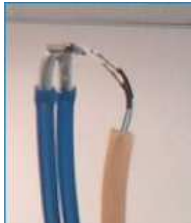
Figure 10. Aluminum tube. The aluminum tube used nitrogen cooled from the vortex tube to cool down and in turn, take heat away from the Peltier cell.
