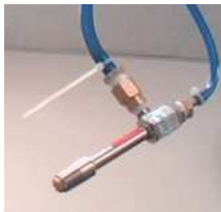
Figure 9. Vortex tube. The vortex tube was used as the heat sink to keep the Peltier cell from overheating.
