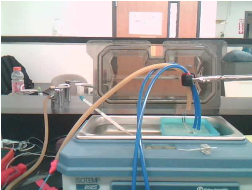
Figure 13. Picture of the testing setup. The agarose is in the blue container in a hot water bath. The water bath has its temperature monitored by a thermometer; thermocouples were used to monitor the temperature of the agarose.
