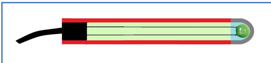
Figure 9: Design Option 3, Attached Thermometer with Circuitry in MedCal
