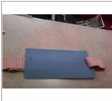
Left: Silicone Mat with imbedded electrode Right: Reusable electrode possibility
