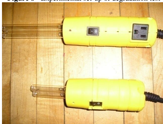
Figure 9 - 9-watt UV light (top) and 5-watt UV light (bottom) used for testing
