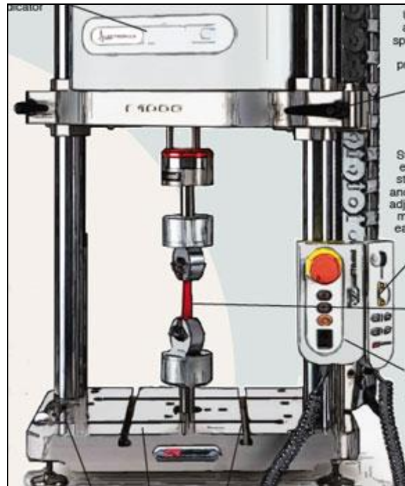
Figure 11 - Experimental set-up of tensile test; example of similar Instron Model 1000 equipment with computer to retrieve data
