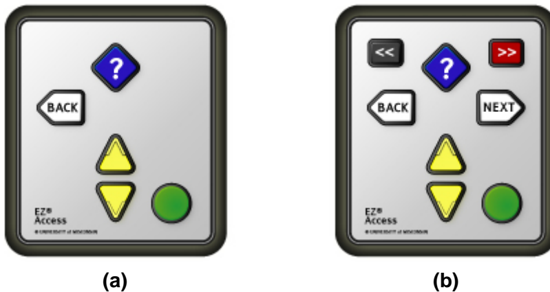
Figure **: (a) 5 button EZ Access keypad [22]. (b) 8 button EZ Access keypad [22].
