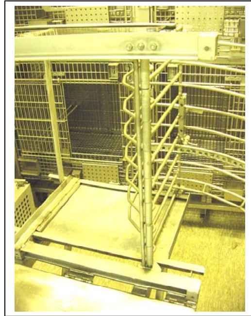
Figure 4 Treatment cage in vertical position. Here the cage is nearly fully closed.
