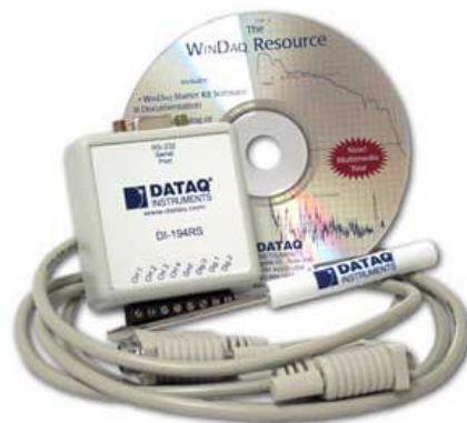
Figure 9. DI-194RS module: serves as an interface between LVDT and PC.
