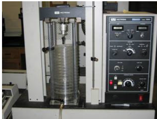
Figure 1. The environmental chamber was designed for use with the Instron 1000 material testing system, located at 1313 Engineering Hall Materials Testing Laboratory.
