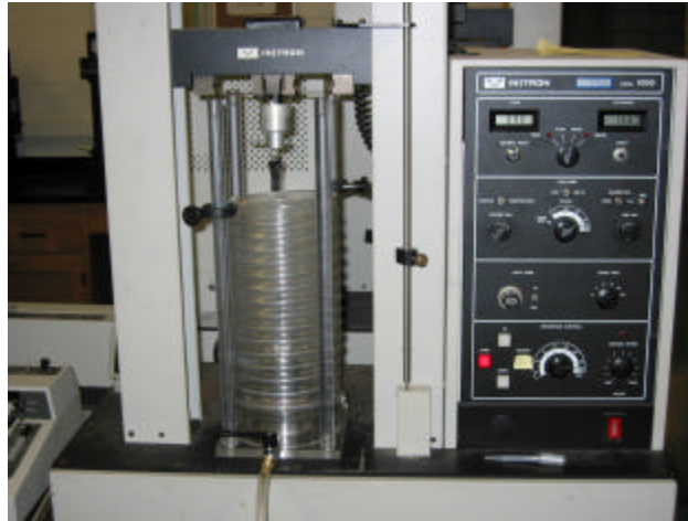
Figure 3. The environmental chamber was designed for use with the Instron 1000 Material Testing System, available at 1313 Engineering Hall Materials Testing Laboratory.
