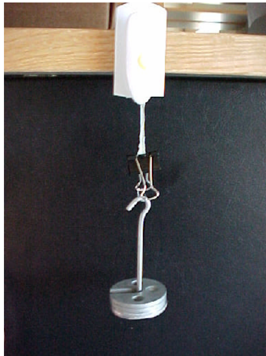
Figure 11. Preliminary Testing system. Binder clips hold the sample, which was loaded from the bottom by weights.
