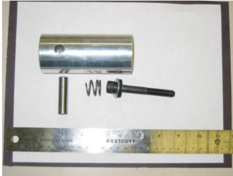
Figure 8 Clockwise from top: aluminum grip adaptor, M10 Cap-head screw with gasket and washer, spring, and steel dowel pin. Ruler is pictured to provide scale.
