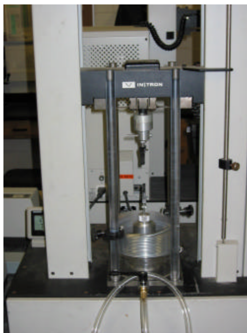
Figure 7. Illustration of environmental chamber on Instron 1000. The chamber's top plate has been removed to allow free travel of the load cell and top grip, and the PVC hose is lowered for orientation of bottom grip within the chamber.
