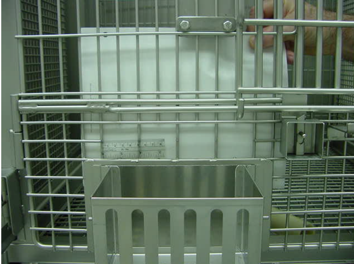
Figure 4: Photograph of “new” cage with a feeding tray mounted directly below large mesh holes (Campbell and Potter, 2002).
