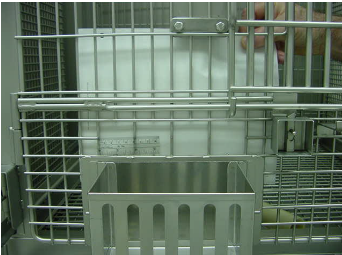
Figure 5: Photograph of “new” cage with a feeding tray mounted directly below large, 4.67-cm. mesh holes (Campbell and Potter, 2002).
