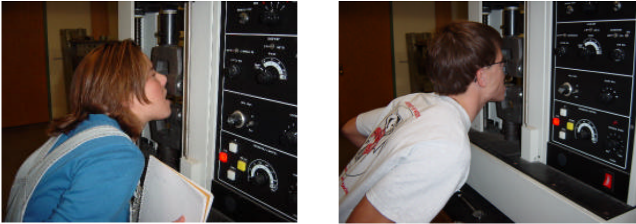
Figure 7. Pictures of both Kathleen (left) and Matt (right) clenching down on L-shaped metal pieces attached to a load cell.
