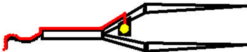
Figure 3: Idea #2, placement of the button on a platform between the arms of the forceps.
