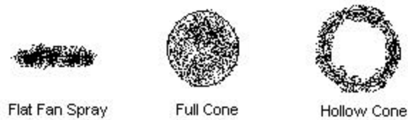
Figure 11: Spray Types. The spray patterns for a flat fan, full cone, and hollow cone are displayed. The full cone spray nozzle will be used.
