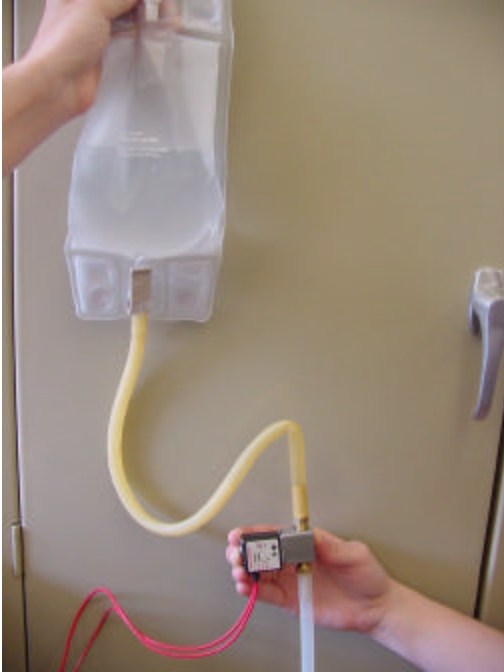
Figure 12: ASCO Red-Hat valve attached to urine bag drainage tubing via barb fitting.
