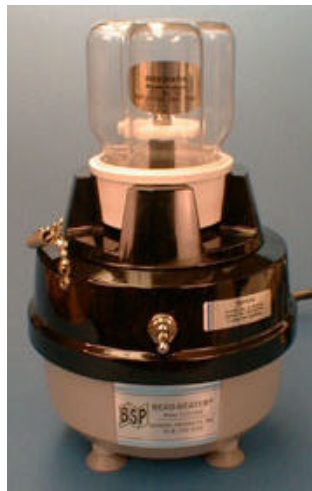
Figure 1: The BeadBeaterä . The top unit spins the metal or glass beads to create collisions with the tissue particles. The collision force breaks apart the tissue. Beads must be cleaned after each use (Meyer, 2002). Image from < http://www.biospec.com >.
