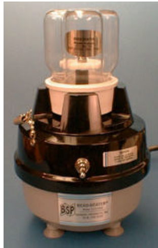
Figure 1. An image of the BeadBeater™ from < http://www.biospec.com >. The top unit spins the metal or glass beads to create collisions with the tissue particles. The collision force breaks apart the tissue. Beads must be cleaned after each use (Meyer, 2002).
