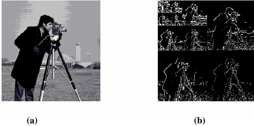
Figure 4: Example of a Two dimensional DWT. (a) shows the original image and (b) shows the scaled DWT coefficients
