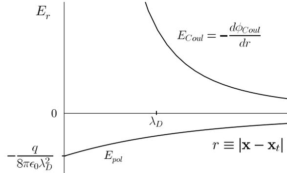
Figure 1.2: Coulomb and polarization radial electric fields around a test particle of charge  $q$  in a plasma. Because the plasma polarization acts to shield out the positive Coulomb electric field, the polarization electric field is negative. The polarization electric field is finite at the origin, decays smoothly with distance away from the test charge, and shields out the Coulomb electric field for separations larger than the Debye length  $\lambda_D$ .
