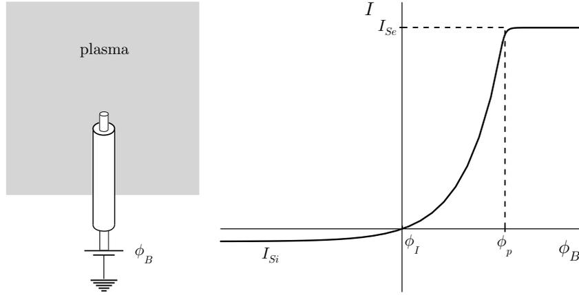
Figure 1.4: Schematic of Langmuir probe inserted into a plasma and its idealized current-voltage characteristics: current  $I$  drawn out of the probe as a function of the bias voltage or potential  $\Phi_B$ . The labeled potentials and currents are:  $\Phi_f$ , floating potential;  $\Phi_p$ , plasma potential;  $I_{Si}$ , ion saturation current;  $I_{Se}$ , electron saturation current.
