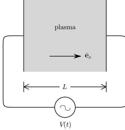
Figure 1.5: Schematic of circuit for imposing an oscillating potential  $\Phi(t) = \Phi_0 \sin \omega_0 t$  across a plasma.
