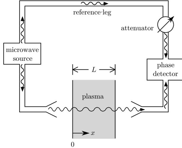
Figure 1.11: Schematic illustration of a microwave interferometer. The electromagnetic wave passing through the plasma has a smaller wavenumber (longer wavelength) than the wave passing through vacuum in the reference leg. Thus, there is a phase shift between the two signals arriving at the detector.
