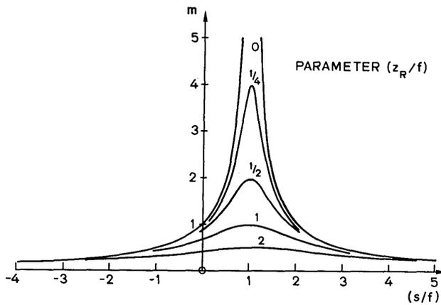
Fig. 5. Graph of magnification for a Gaussian beam vs normalized object distance, with normalized Rayleigh range of the input beam as the parameter.
