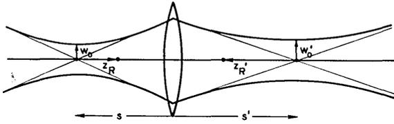
Fig. 3. Geometry of the imaging of a Gaussian beam by a lens shown for the case of a positive lens and real object and image waists.
