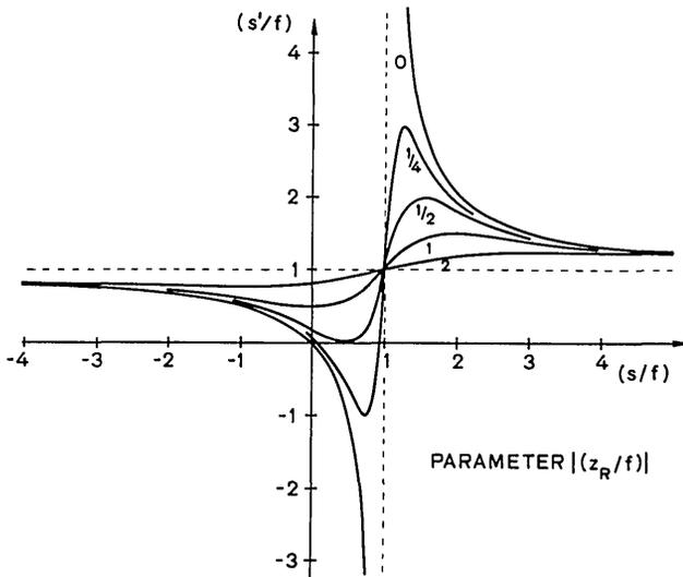
Fig. 4. Cartesian plot of the lens formula for Gaussian beams showing normalized image distance vs normalized object distance, with normalized Rayleigh range of the input beam as the parameter.
