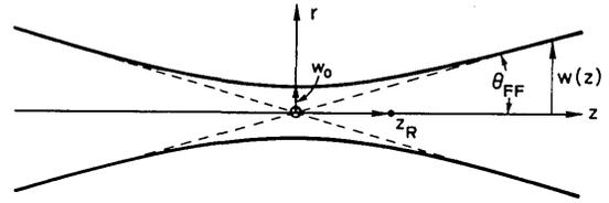
Fig. 2. Geometry of a spherical Gaussian beam.
